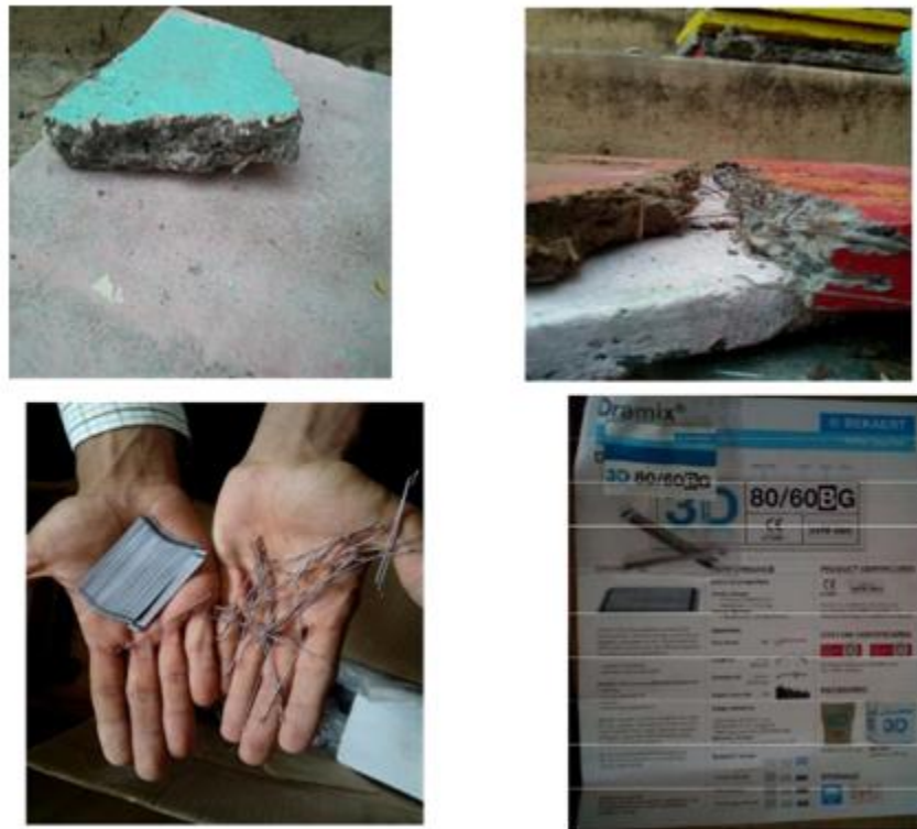
Fig.3 Steel fibre reinforced tiles
